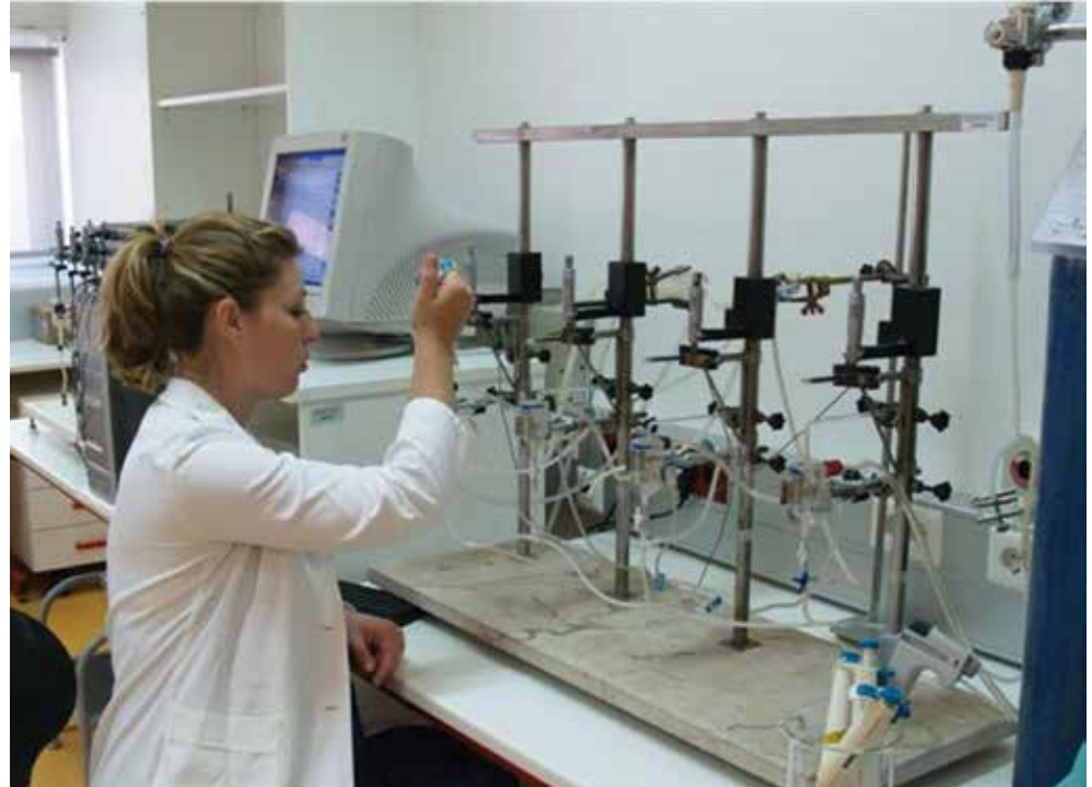
Slika 2. Sustav za izolirane krvožilne prstenove. Figure 2. System for isolated blood vessel rings.
